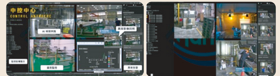
CCTV+AI smoke detection system
